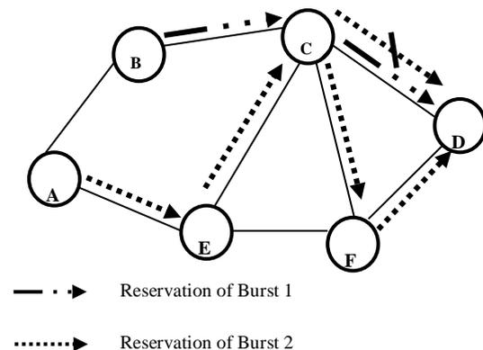
Figure 2 Conceptual view of deflection routing
