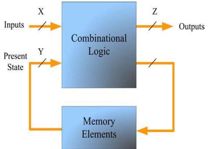
Fig. 1.1 General Diagram of Mealy machine
