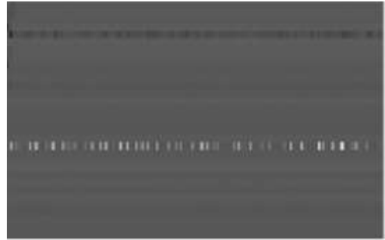
Figure-6: Final acquired image after the sliding rectangle algorithm on a homogeneous medium used as phantom
