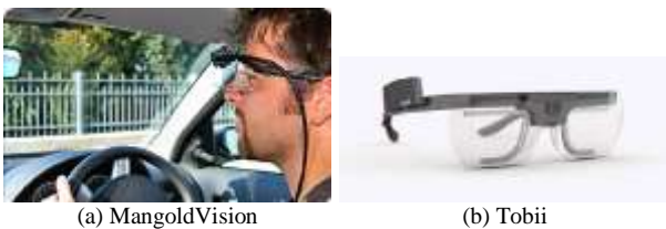
Figure 3. MangoldVision in (a) and Tobii in (b) designs wearable glasses that appends a camera to estimate the pupil position.
