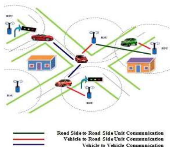
Fig. 2: Vehicular network architecture
