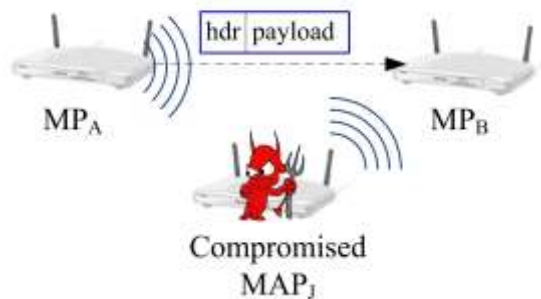
Fig. 3(a) A data-selective jamming attack
