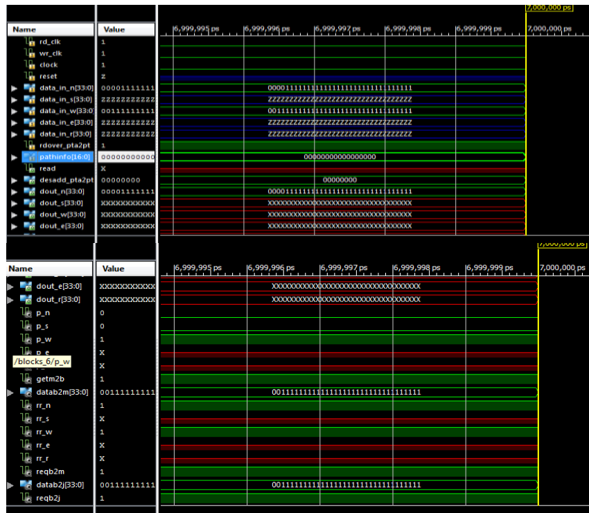
Figure 10: Simulation Report of 6 blocks( Input port, Header Modifier, Junction and Resource Control, Path Table Arbiter, Arbiter and Crossbar) have been interfaced together. The inputs are given to data_in pin in any direction required and the output is obtained from data_out in the same direction as the input given.
