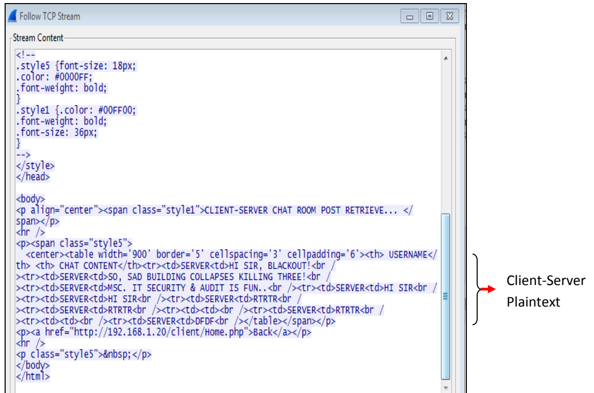
Figure 17: Plaintext Client-Server Communication
