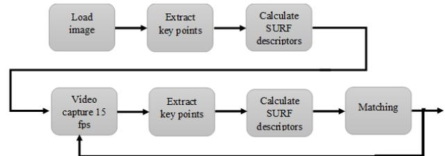
Figure. 5: object detection algorithm in real time
