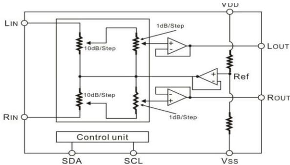
to 1. If CODE1 or CODE2 is connected to the Ground, it is set to 0. Data byte Description. Every byte transmitted to SDA line consist of 8 bits. Each byte must be followed by acknowledge bit. The MSB is transmitted first.
