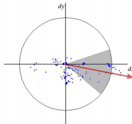
Figure. 3: Orientation assignment: A sliding orientation window of size  $\pi/3$  detects the dominant orientation of the Gaussian weighted Haar wavelet responses at every sample point within a circular neighbourhood around the interest point. [11]
