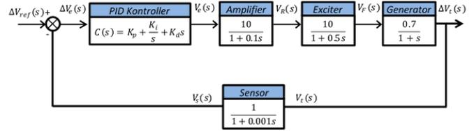
Figure 3. AVR system diagram block with PID controller
