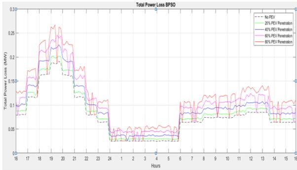
Figure 6. Total power loss system using BPSO algorithm
