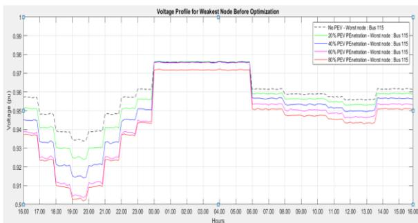
Figure 5. Voltage profile for weakest node before optimization
