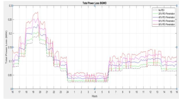
Figure 9. Total power loss system using BGWO algorithm
