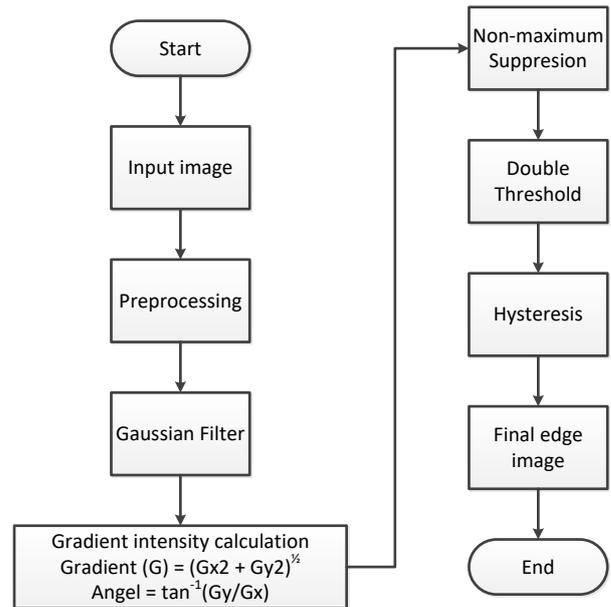
Figure 2. Canny edge detection feature extraction flowchart
