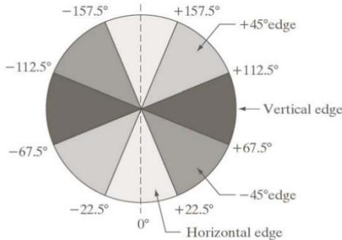
Figure 4. Range of angle direction of non-maximum suppression
