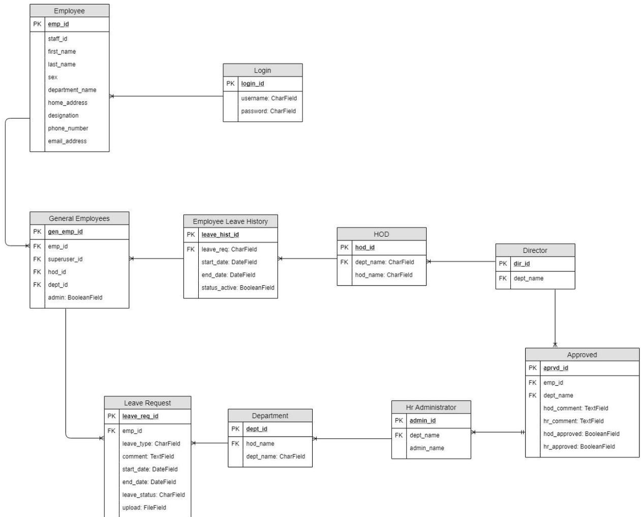
Figure 9. Entity Relationship Diagram for Leave management System.
