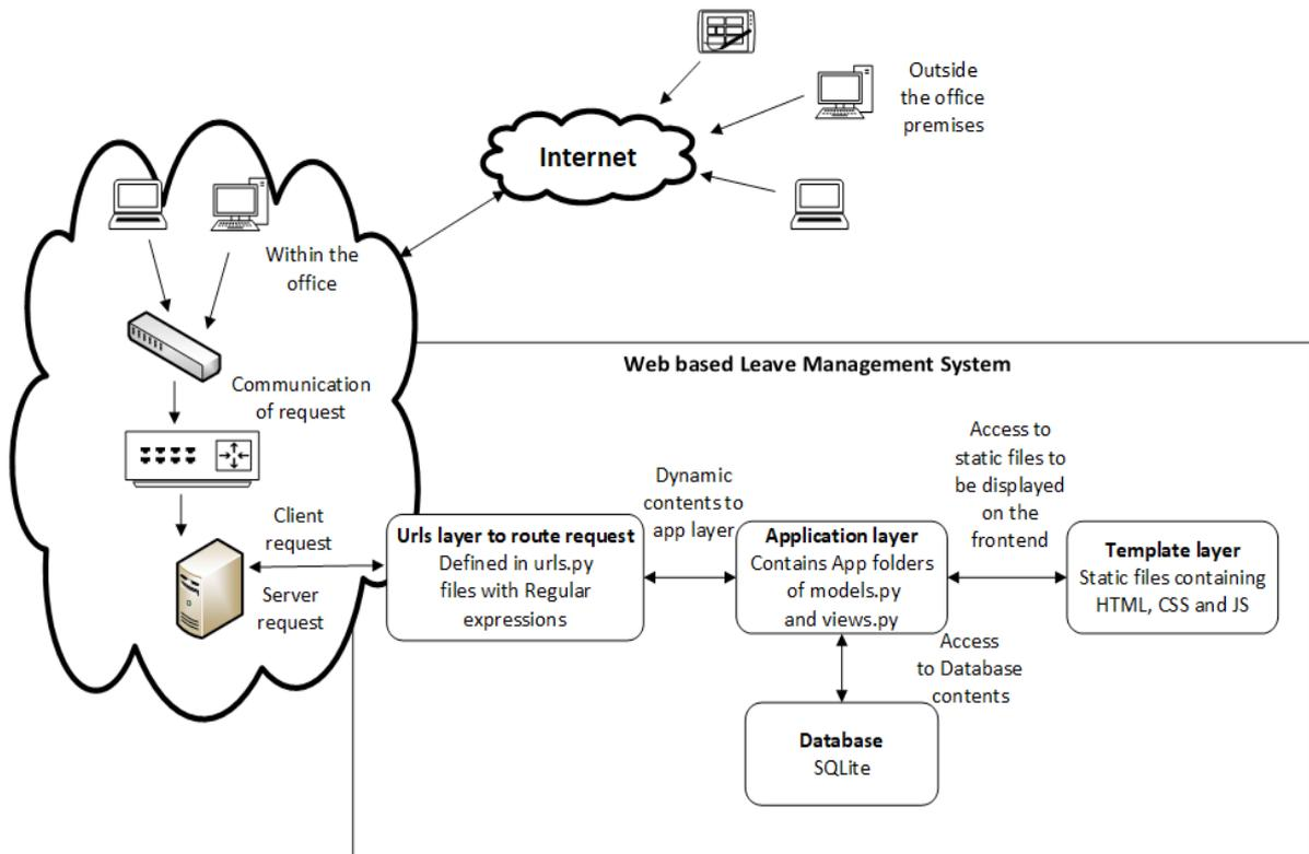
Figure 4: System Architecture for the Leave Management System
