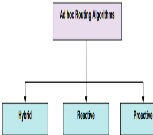
Figure 3: Generalized MANETs Routing Protocols Classification [17]
