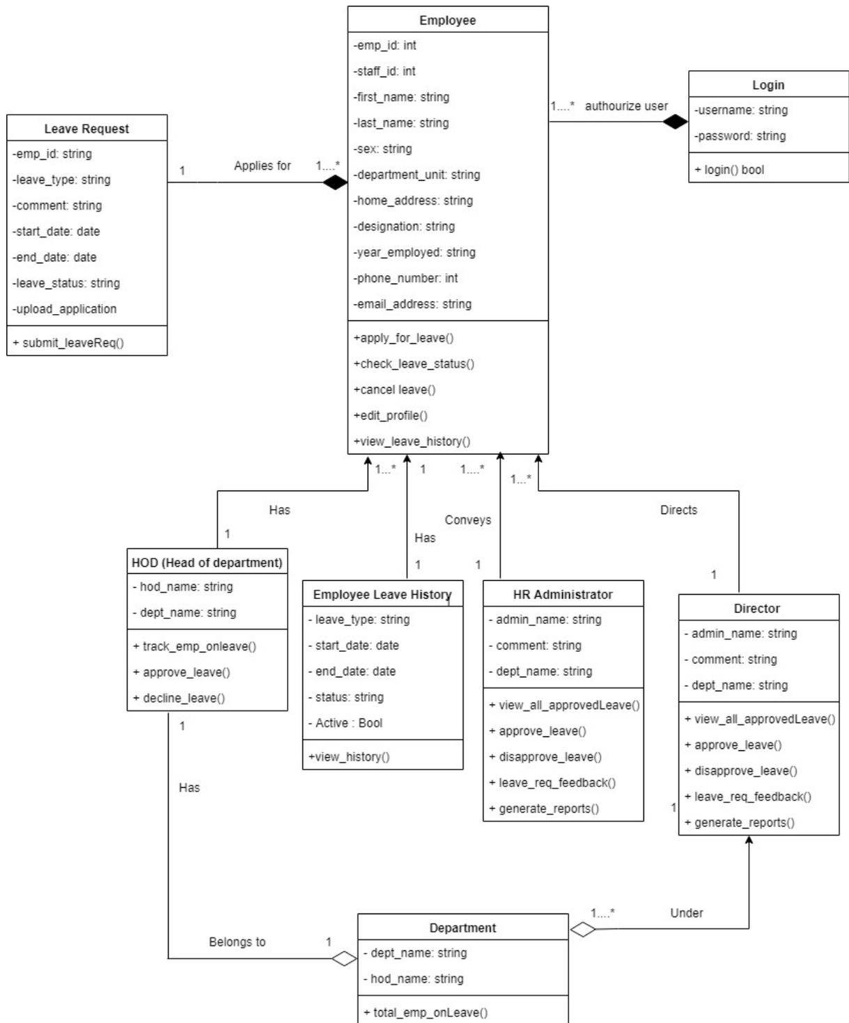
Figure 7. Class Diagram for the Leave Management System
