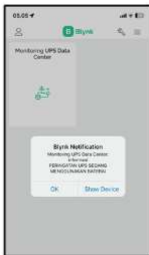
Figure 4. Notification When UPS Is Using Battery
