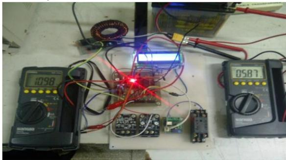
Figure 10. The test results of the Buck Converter circuit to reduce the voltage
