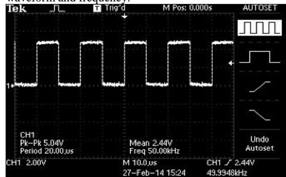
Figure 8. Example of 50% PWM waveform and 50 kHz frequency
