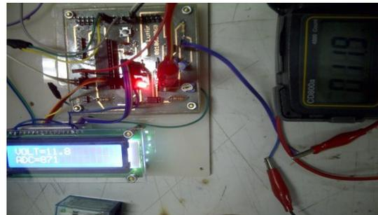
Figure 12. Test result of voltage sensor circuit
