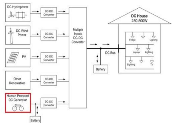
Figure 1. The main system in the DC House electrical installation.
