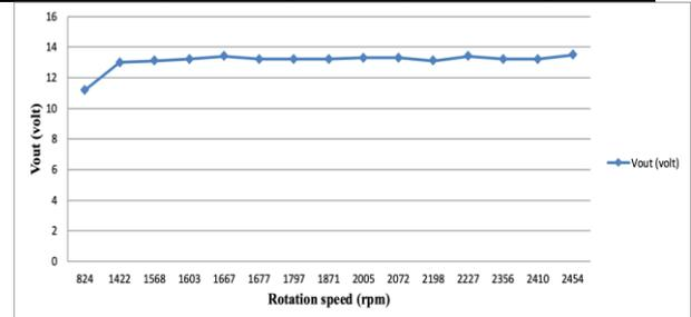
Figure 14. Graph of output voltage versus rotation speed
