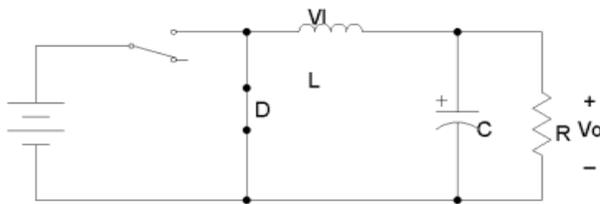
Figure 3. Buck converter circuit when switch is OFF
