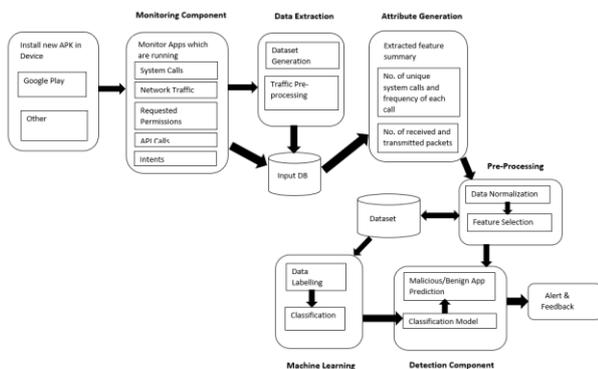
Figure 1 Proposed Architecture of Android Vulnerability Detection
