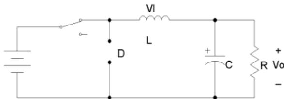
Figure 2. Buck converter circuit when switch is ON
