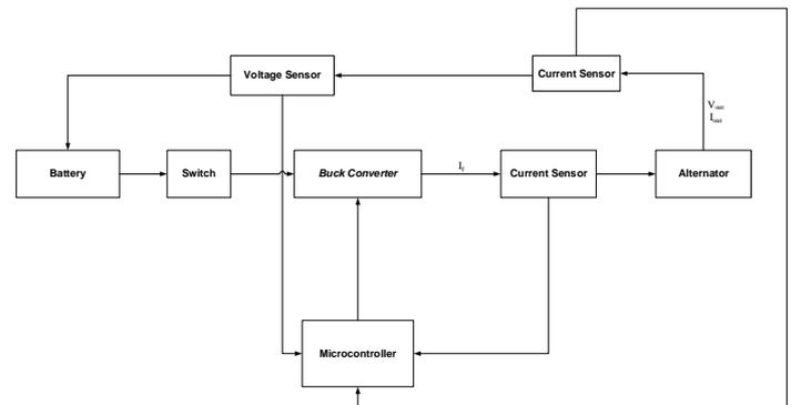
Figure 4. Block Diagram of Charge Controller System
