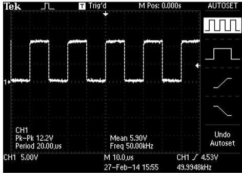
Figure 9. Example of MOSFET driver output waveform with 50% duty cycle
