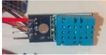
Fig.2 DHT11 Temperature and Humidity Sensor
