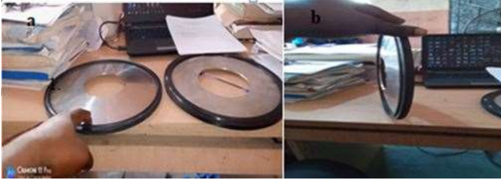
Fig 1: (a)Picture of the Concentric Orifice Plate, (b) Side Picture of the Concentric Orifice Plate
