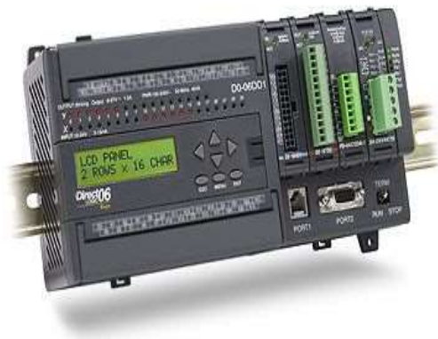
Figure 1 Example of a Type of PLC
