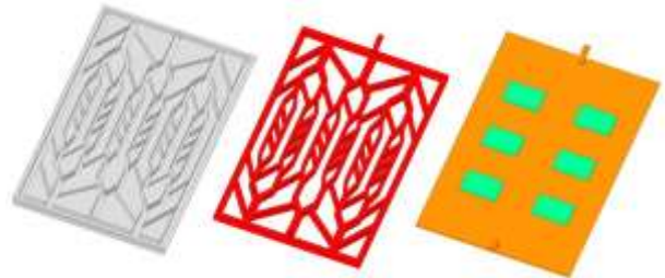
Figure 1 IGBT Liquid Cooling Channel Model
