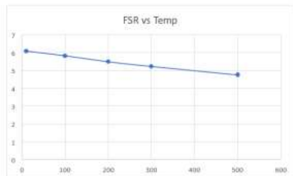
Fig. 3.2 Variation of FSR with temperature in a Si single ring resonator
