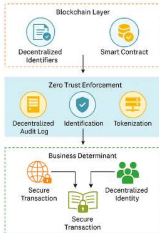
Figure 4: Proposed integrated ZTA-Blockchain framework for cross-border digital identity and transaction verification
