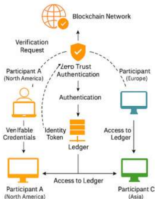
Figure 5: Workflow of a real-time blockchain-based ZTA transaction validation across three financial jurisdictions
