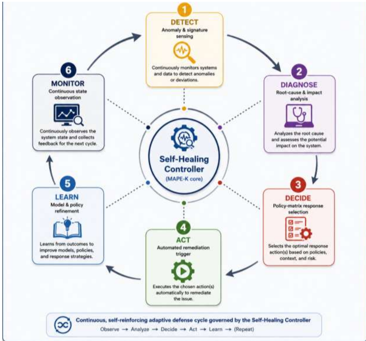
Fig. 3: Self-Healing Feedback Control Loop. The six-phase cycle (Detect - Diagnose - Decide - Act - Learn - Monitor) forms a continuous, self-reinforcing adaptive defense mechanism governed by the Self-Healing Controller.
