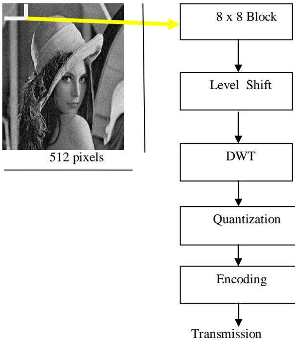
Figure 1. JPEG Algorithm block diagram
