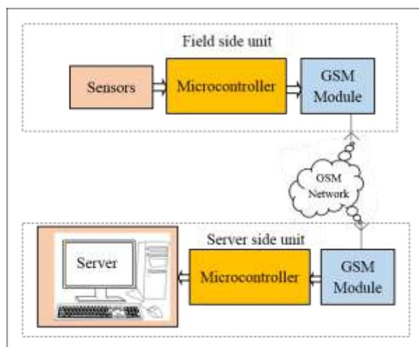
Figure. 1 The system functional block diagram.
