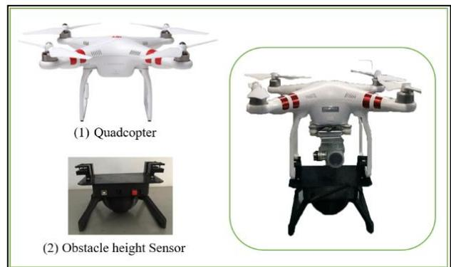
Figure 8. The Transmitter of Obstacle Height Monitoring System
