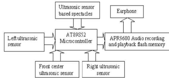
Figure 2.2: Ultrasonic Spectacles and Waist-belt for Visually Impaired and Blind Person
