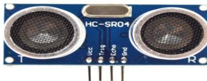
Fig .3.2: HC-SR04 Ultrasonic Sensors
