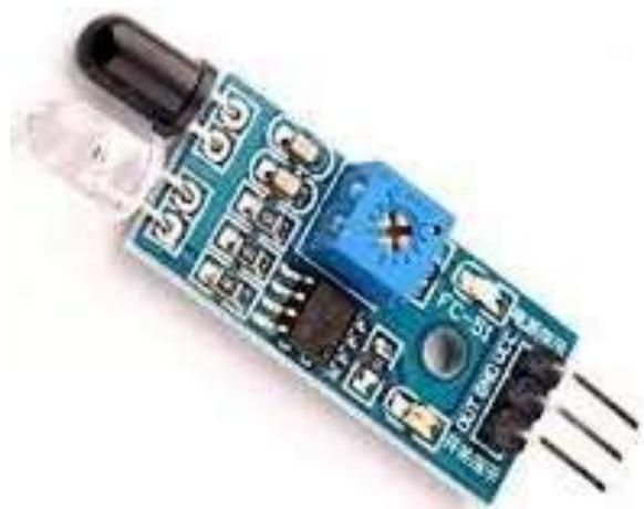
Figure 1 Infrared transceiver module.
